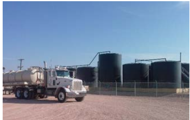
Figure 7: Truck unloading into tank battery for salt water / oil storage and separation
